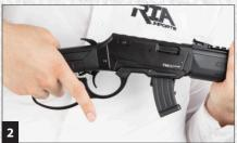
**3)** When the lever is completely closed, the lever will push the safety and changes it to off position.
