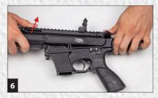
7) With the pin punch still in the upper receiver, use your thumb to cover the back of the guide rod or place the upper receiver against a hard flat surface, preferably a table or work bench. Slowly retract the pin punch from the receiver and slowly move your thumb away, or lift the upper assembly up, allowing the main spring to decompress.
