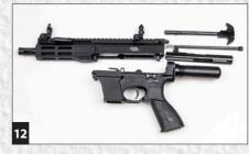
1) Insert the charging handle into the upper receiver and align the charging handle ears with the 2 notches cut out in the receiver.
