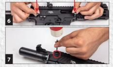
NOTE: Perform a function test by pulling back on either side or rear charging handle. Action should move freely and smoothly. If the action is not moving freely reverse the assembly steps and reassemble until it is.
